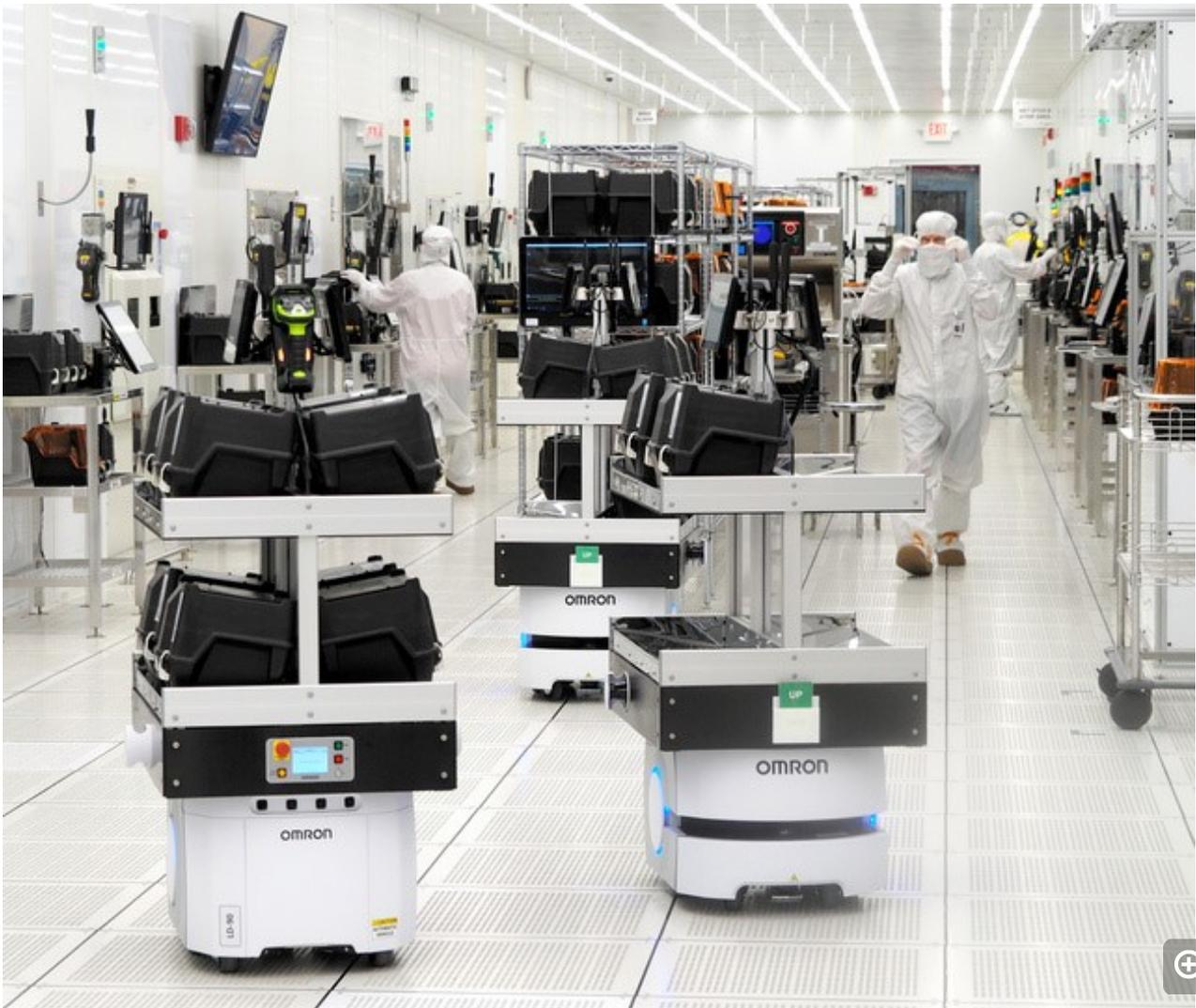
An OMRON robot carrying wafers moves around with clean-wearing workers at the semiconductor manufacturing plant of Polar Semiconductor, a subsidiary of Sanken Electric Co. in the U.S. (Photo: Naoatsu Aoyama, Bloomington, Minnesota, U.S.A., May 26)
